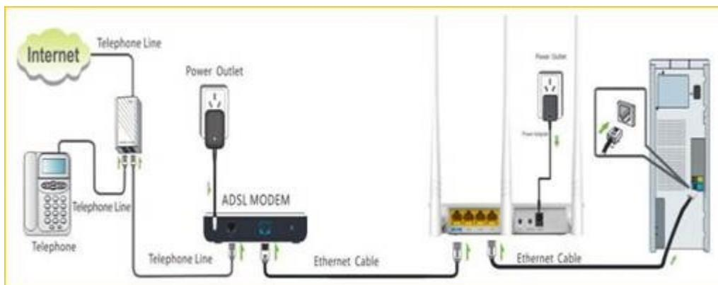
**Note:** after connection the **sys** light should be blinking, the **WLAN** light should be on or blinking, the **WAN** light should be on or blinking.
