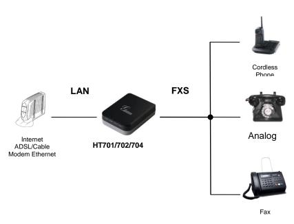
FIGURE 2: HT70X CONNECTION DIAGRAM
